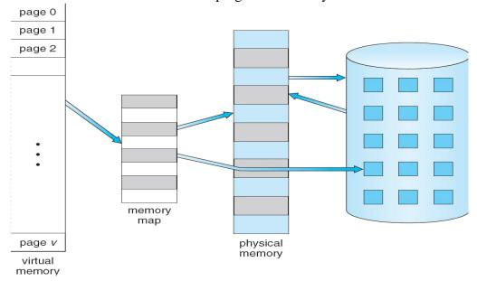
Fig. Diagram showing virtual memory that is larger than physical memory.
