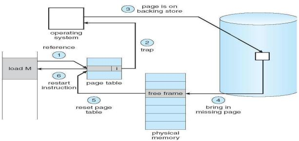
Fig. Steps in handling a page fault
