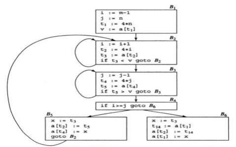
Fig. 5.3 B5 and B6 after common subexpression elimination
