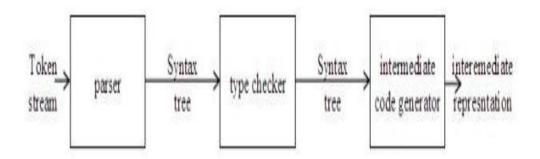
A type checker verifies that the type of a construct matches that expected by its context. For example: arithmetic operator mod in Pascal requires integer operands, so a type checker verifies that the operands of mod have type integer. Type information gathered by a type checker may be needed when code is generated.
