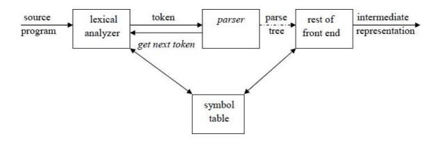
Fig . 4.1: position of parser in compiler model.
