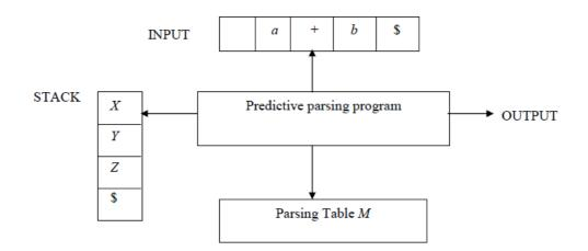
The table-driven predictive parser has an input buffer, stack, a parsing table and an outputstream.
