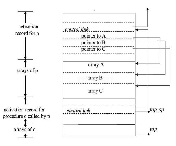
Access to dynamically allocated arrays
