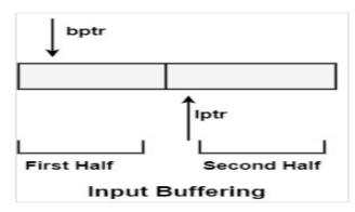
**Sentinels** – Sentinels are used to making a check, each time when the forward pointer is converted, a check is completed to provide that one half of the buffer has not converted off. If it is completed, then the other half should be reloaded.
