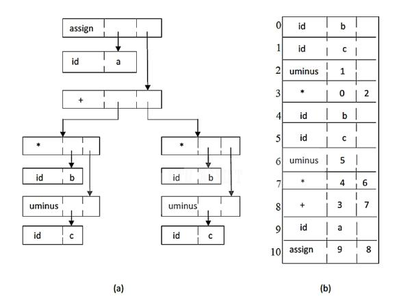
In (*a*<sup>+</sup>, each node is represented as a record with a field for its operator and additional fields for pointers to its children.
