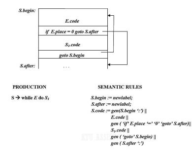
The function *newtemp* returns a sequence of distinct names t1, t2,.... in respose of successive calls. Notation gen(x := 'y + 'z is used to represent the three address statement x := y + z.
