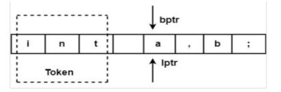
A buffer can be divided into two halves. If the look Ahead pointer moves towards halfway in First Half, the second half is filled with new characters to be read. If the look Ahead pointer moves towards the right end of the buffer of the second half, the first half will be filled with new characters, and it goes on.
