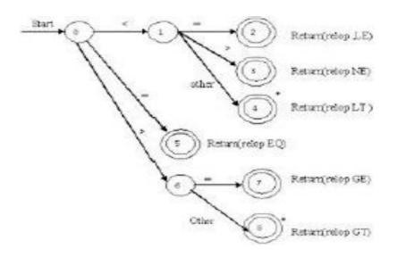
Fig. 3.3: Transition diagram of Relational operators
