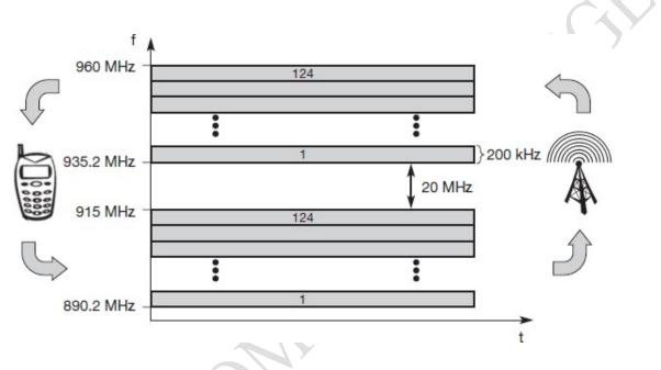
• The two directions, mobile station to base station and vice versa are now separated using different frequencies. This scheme is then called frequency division duplex (FDD).
