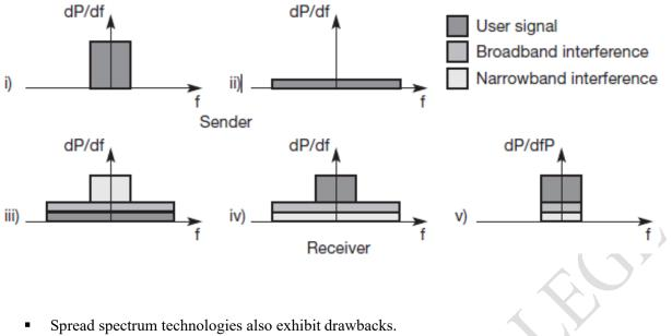
• The effect of spread spectrum if a secret code is used for spreading.
