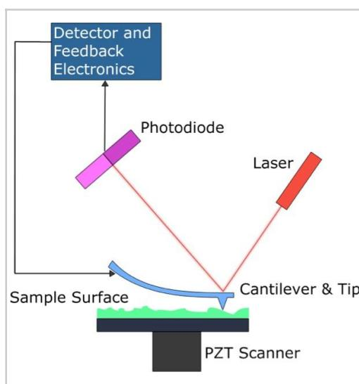
The tip is moved across the sample many times. This is why these are called “scanning” microscopes. A computer combines the data to create an image
