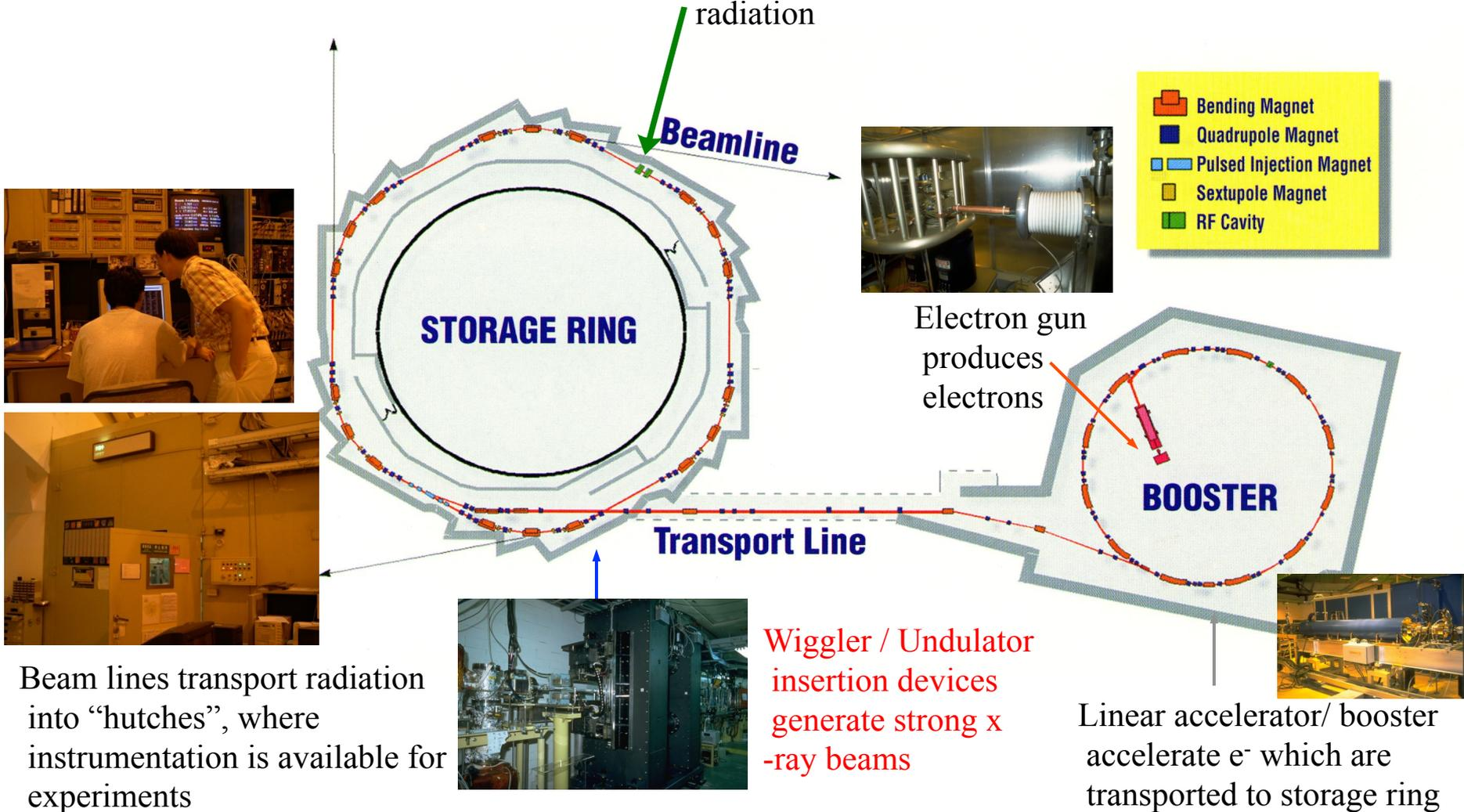
Beam lines transport radiation into “hutches”, where instrumentation is available for experiments
