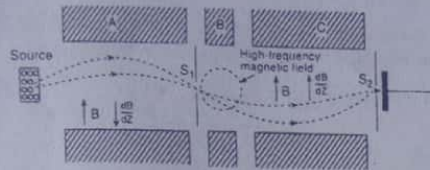
Fig. 1.3 Rabi's method of determining nuclear magnetic moment
