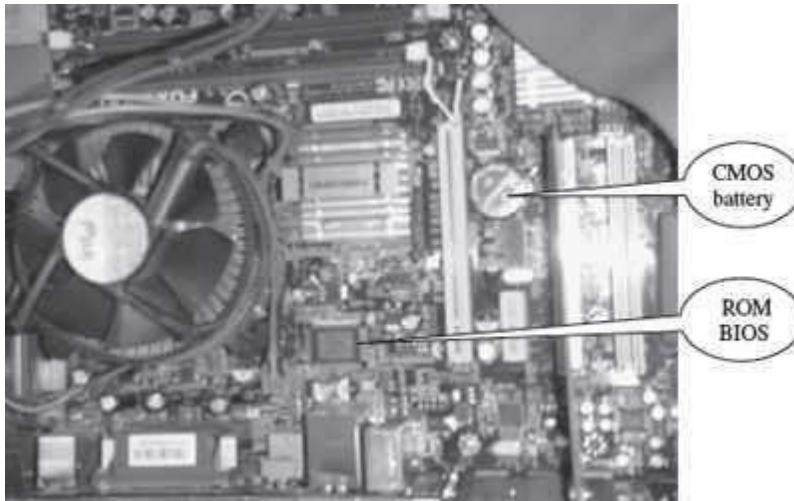
Figure 3.5 ROM BIOS and CMOS battery on a motherboard
