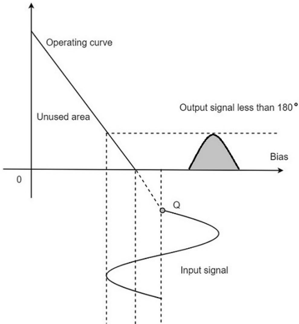
This kind of biasing gives a much improved efficiency of around 80% to the amplifier, but introduces heavy distortion in the output signal. Using the class C amplifier, the pulses produced at its output can be converted to complete sine wave of a particular frequency by using LC circuits in its collector circuit.
