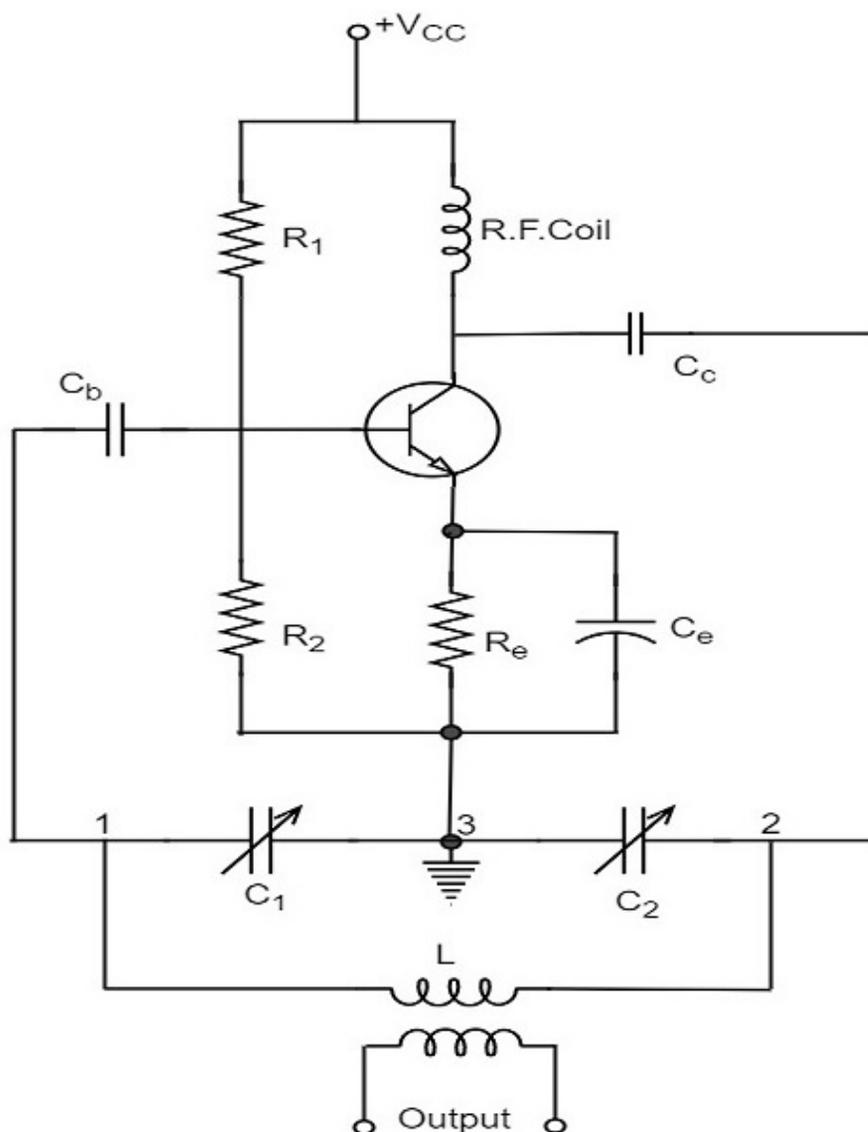
The resistors  $R_1$ ,  $R_2$  and  $R_e$  provide necessary bias condition for the circuit. The capacitor  $C_e$  provides a.c. ground thereby providing any signal degeneration. This also provides temperature stabilization.
