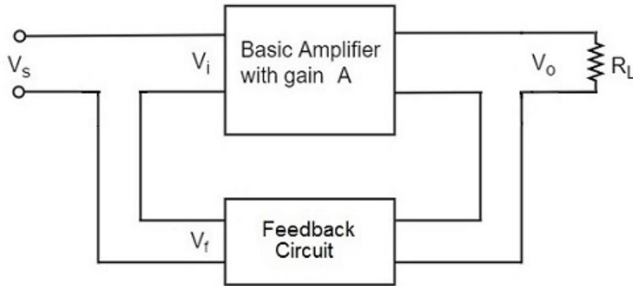
As the feedback circuit is connected in series with the output and the input as well, both the output impedance and the input impedance are increased.
