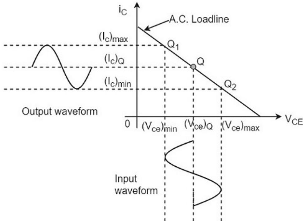
The output characteristics with operating point Q is shown in the figure above. Here  $(I_c)_Q$  and  $(V_{ce})_Q$  represent no signal collector current and voltage between collector and emitter respectively. When signal is applied, the Q-point shifts to  $Q_1$  and  $Q_2$ . The output current increases to  $(I_c)_{max}$  and decreases to  $(I_c)_{min}$ . Similarly, the collector-emitter voltage increases to  $(V_{ce})_{max}$  and decreases to  $(V_{ce})_{min}$ .
