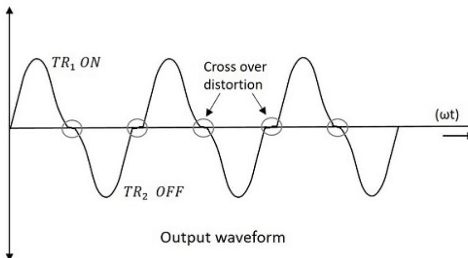
The above figure clearly shows the cross over distortion which is prominent in the output waveform. This is the main disadvantage. This cross over distortion effect also reduces the overall peak to peak value of the output waveform which in turn reduces the maximum power output. This can be more clearly understood through the non-linear characteristic of the waveform as shown below.
