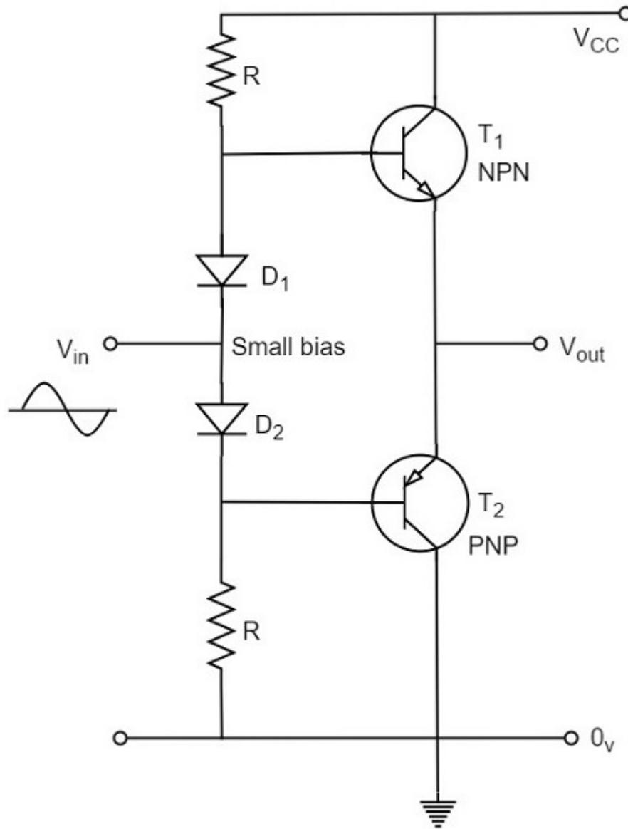
Therefore, in class AB amplifier design, each of the push-pull transistors is conducting for slightly more than the half cycle of conduction in class B, but much less than the full cycle of conduction of class A.
