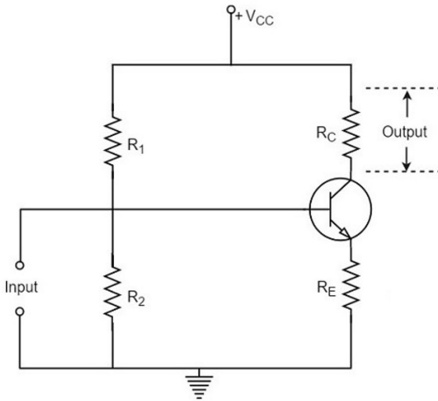
When a weak input signal is given to the base of the transistor as shown in the figure, a small amount of base current flows. Due to the transistor action, a larger current flows in the collector of the transistor. (As the collector current is  $\beta$  times of the base current which means  $I_C = \beta I_B$ ). Now, as the collector current increases, the voltage drop across the resistor  $R_C$  also increases, which is collected as the output.
