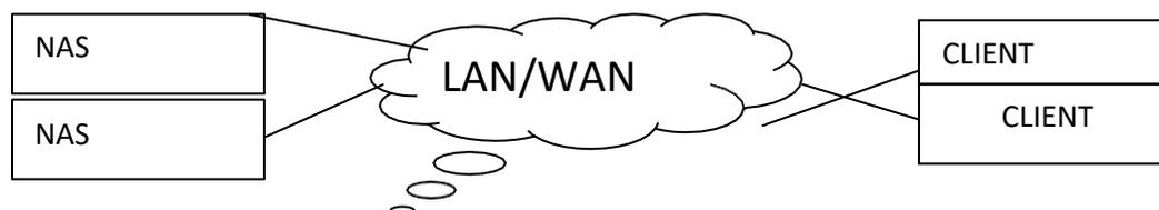
NAS provides a convenient way for all the computers on a LAN to share a pool of storage with the same ease of naming and access enjoyed with local host attached storage .but it tends to be less efficient and have lower performance than direct attached storage.
