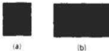
Turning a square (a) Into a rectangle (b) with scaling factors s_x = 2 and s_y = 1 .
