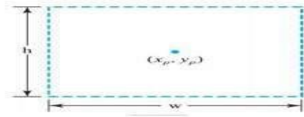
Figure 20-2 A pick window with center coordinates (x_p, y_p) , width w , and height h
