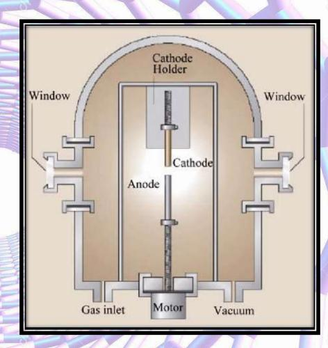
**❖For** growing SWNTs, graphite electrodes are impregnated with metalcatalysts like Co, Cu, and Fe.
