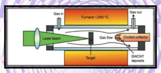
In this technique, the SWNTs are formed as ropelike crystallites, 5-20 nm in diameter and tens to hundreds of micrometers in length.
