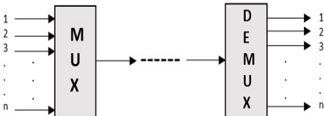
Multiplexing and Demultiplexing
