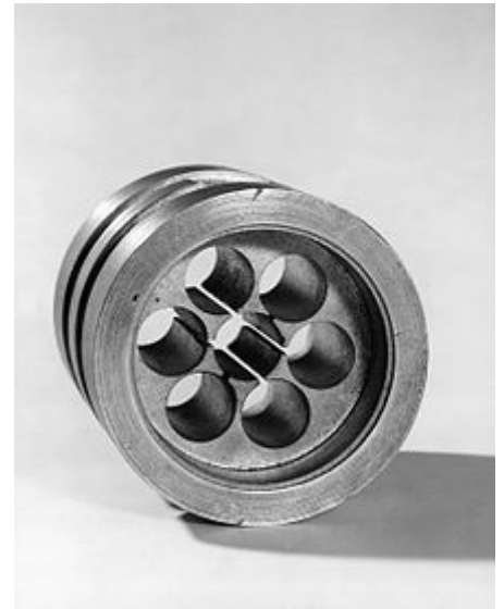
The cavity magnetron developed by John Randall and Harry Boot in 1940 at the University of Birmingham England
