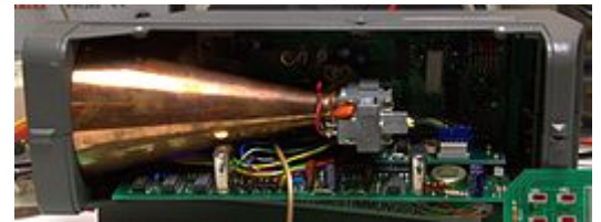
Disassembled radar speed gun. The grey assembly attached to the end of the copper-colored horn antenna is the Gunn diode which generates the microwaves.
