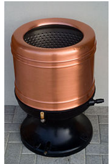
German laundry centrifuge to extract water from laundry. The advent of automatic washing machines with spin cycles made such specialized appliances largely obsolete by the 1970s.
