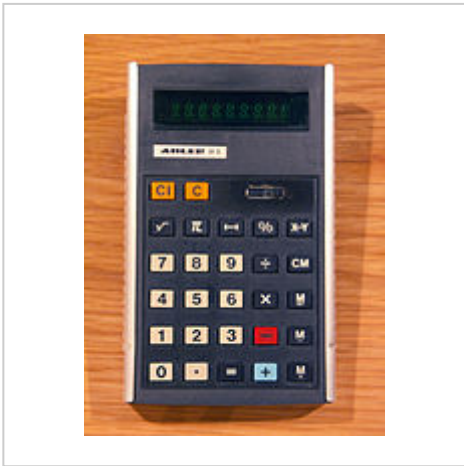
Adler 81S pocket calculator with vacuum fluorescent display (VFD) from the mid-1970s.
