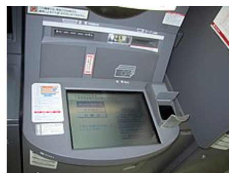
A BTMU ATM with a palm scanner (to the right of the screen)
