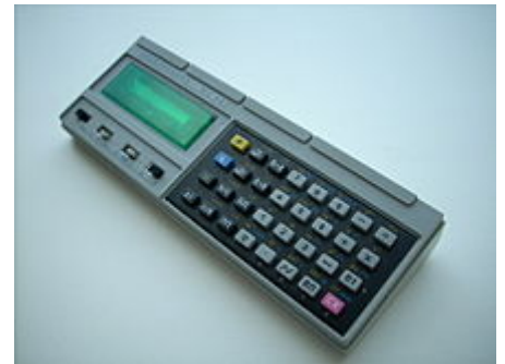
The Elektronika MK-52 was a programmable RPN-style calculator that accepted extension modules; it was manufactured in the Soviet Union from 1985 to 1992
