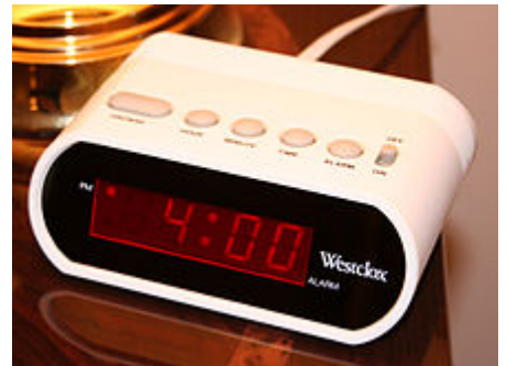
Basic digital alarm clock without a radio. The mark in the top-left of the display indicates that the time is 4:00pm, not 4:00am.
