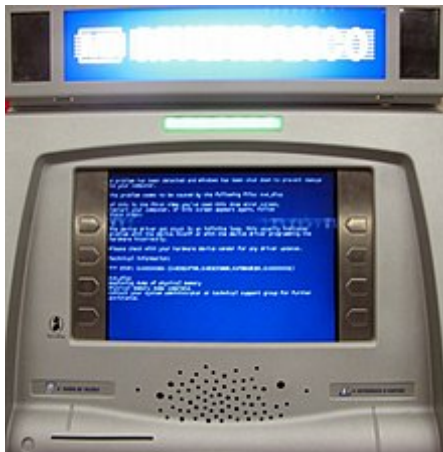
An ATM running Microsoft Windows that has crashed due to a peripheral component failure
