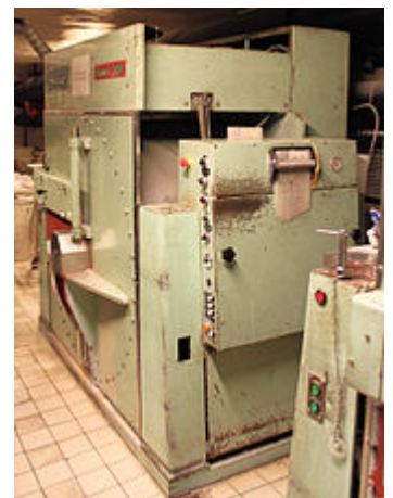
A 1980s Belgian 90 kg load industrial washer (horizontal axis, front load)
