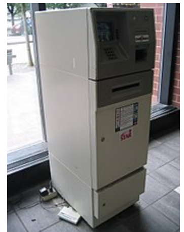
A Diebold 1063ix with a dial-up modem visible at the base
