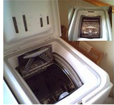
European top loader with horizontal axis rotating drum (2008)
