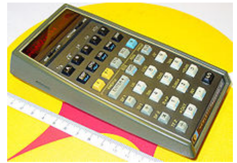
The HP-65, the first programmable pocket calculator (1974)
