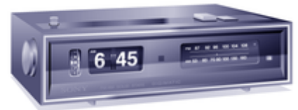
A 1969 radio alarm clock (Sony Digimatic 8FC-59W) with an early mechanical-digital display
