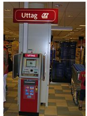
Smaller indoor ATMs dispense money inside convenience stores and other busy areas, such as this off-premises Wincor Nixdorf mono-function ATM in Sweden.
