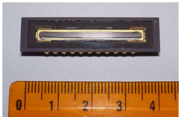
CCD MN8051 Matsushita CCD side, monochrome 2048-bit linear sensor +cm (centimeters)
