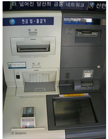
A South Korean ATM with mobile bank port and bar code reader
