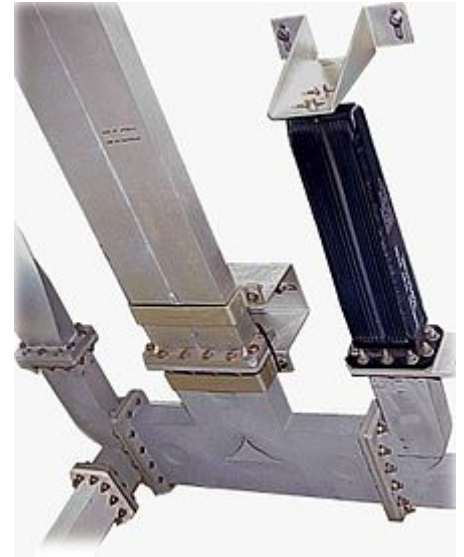
Waveguide is used to carry microwaves. Example of waveguides and a diplexer in an air traffic control radar
