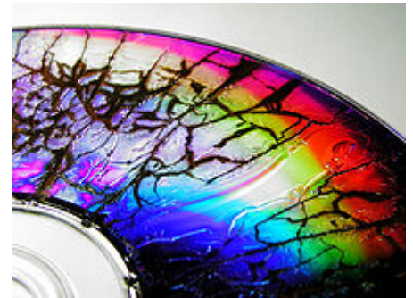
A microwaved DVD-R disc showing the effects of electrical discharge through its metal film
