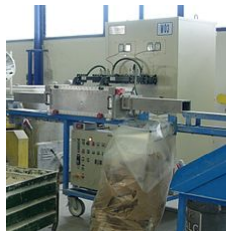
Microwaves are widely used for heating in industrial processes. A microwave tunnel oven for softening plastic rods prior to extrusion.
