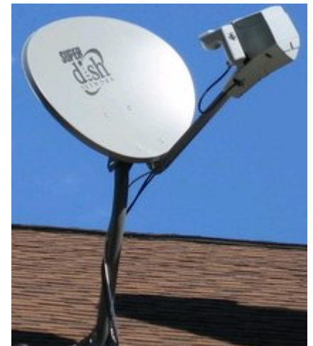
A satellite dish on a residence, which receives satellite television over a K_u band 12–14 GHz microwave beam from a direct broadcast communications satellite in a geostationary orbit 35,700 kilometres (22,000 miles) above the Earth.
