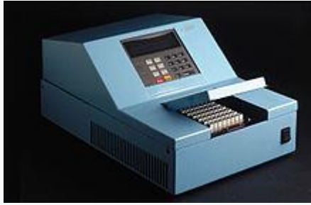
"Baby Blue", a 1986 prototype machine for doing PCR
