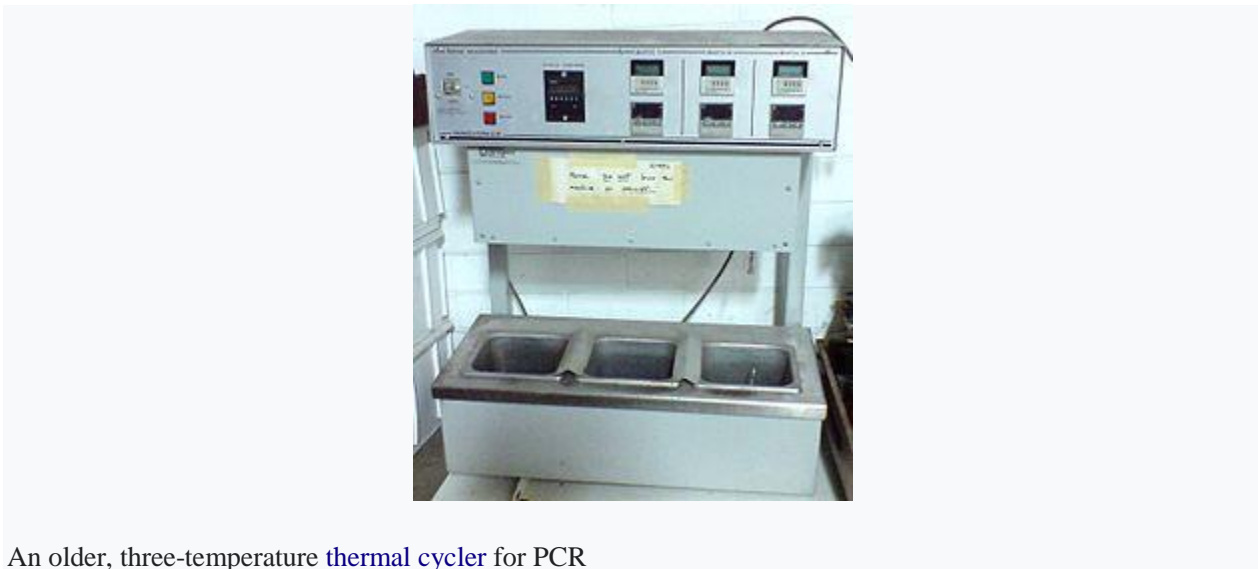
An older, three-temperature thermal cycler for PCR
