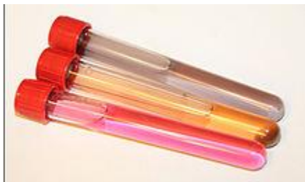
Reduced forms of Cyanocobalamin, with a Co(I) (top), Co(II) (middle), and Co(III) (bottom)
