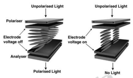
Fig. 11: Operation of a twisted nematic cell
