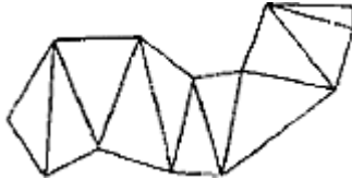
Fig. 4.7: -A triangle strip formed with 11 triangle connecting 13 vertices
