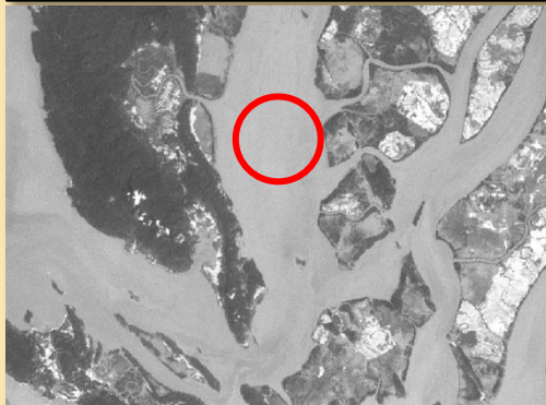
TM Band 1: High reflectance in water TM Band 4: High reflectance in vegetation TM Band 7: High reflectance in bare land (soil)
