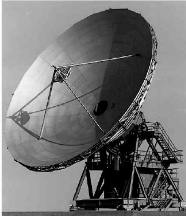
Figure 6b.7: Double Reflector Cassegrain Antenna.
