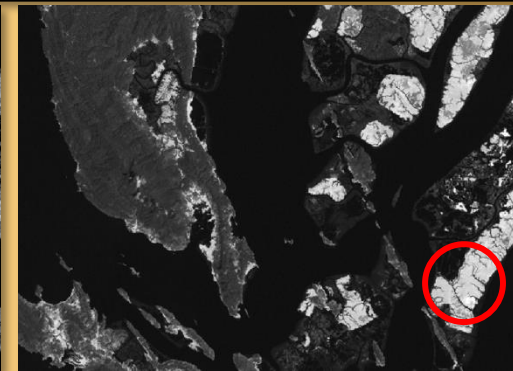
TM Band 1: High reflectance in water TM Band 4: High reflectance in vegetation TM Band 7: High reflectance in bare land (soil)
