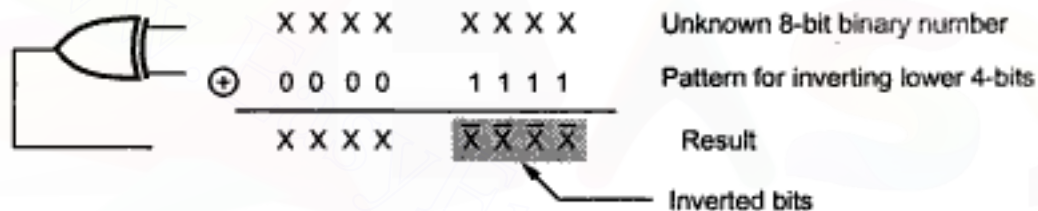
Fig. 3.2 Inversion of part of a number using XOR operation
