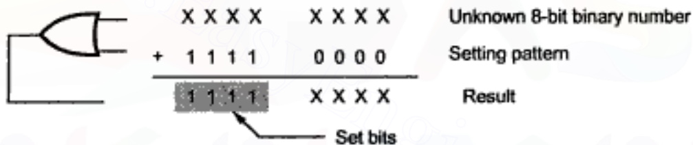
Fig. 8.4 Setting bit/s using OR operation
