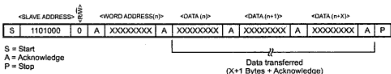
Fig. 15.15 Data write - slave receiver mode
