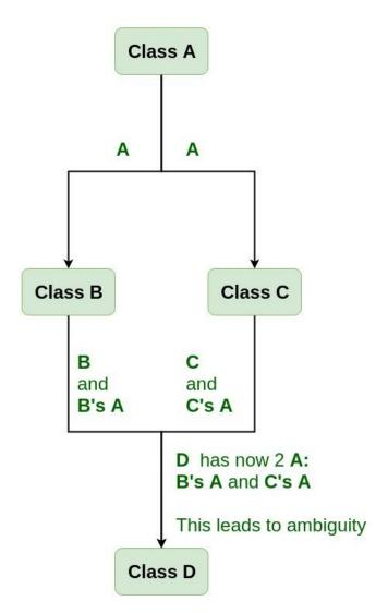
As we can see from the figure that data members/function of class **A** are inherited twice to class **D**. One through class **B** and second through class **C**. When any data / function member of class **A** is accessed by an object of class **D**, ambiguity arises as to which data/function member would be called? One inherited through **B** or the other inherited through **C**. This confuses compiler and it displays error.
