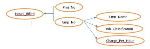
In the above diagram **Hours\_Builled** depends on Project\_No and Emp\_No but the remaining non key fields (Emp\_Name,Job\_Class,Charge\_per\_Hour)depends on Emp\_No this situation is an example of 2<sup>nd</sup> normal form .Hence the relation 3 is divided into 2 relations.
