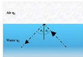
Figure. Total Internal Reflection (TIR), an incident beam of light with angle \theta_1 , is passing through a media with refractive index \eta_1 , the beam reflects back at angle \theta_2 , when the refractive index of the medium changes to a value \eta_2 .
