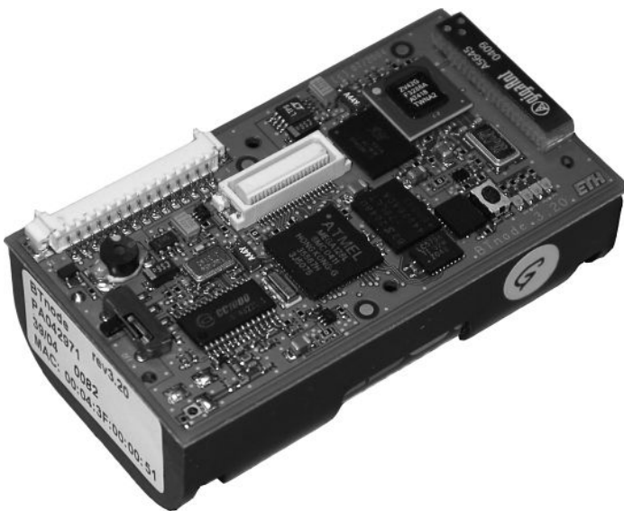
Figure 2.14 Btnode. Reproduced by permission of Jan Beutel, ETH Zurich
