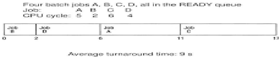
(Figure 4.6) Timeline for job sequence B, D, A, C using the SJN algorithm. © Cengage Learning 2014
