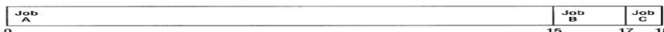
(figure 4.6) Timeline for job sequence A, B, C using the FCFS algorithm. © Cengage Learning 2014
