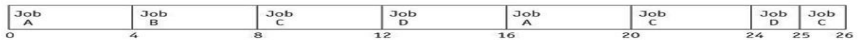
(figure 4.11) Timeline for job sequence A, B, C, D using the preemptive round robin algorithm with time slices of 4 ms. © Cengage Learning 2014
