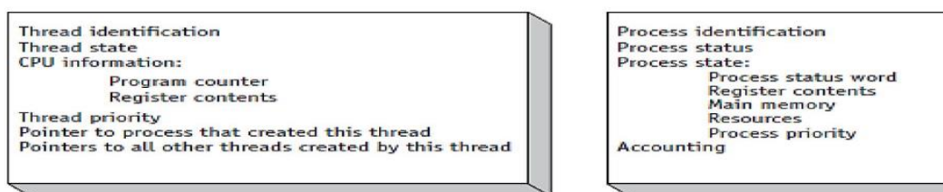
(figure 4.4) Comparison of a typical Thread Control Block (TCB) vs. a Process Control Block (PCB). © Cengage Learning 2014
