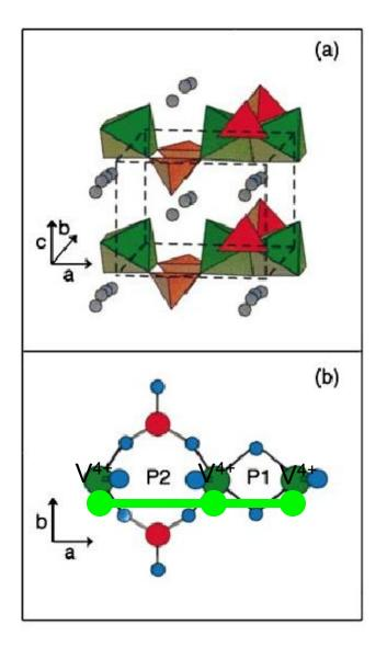
The use of neutron scattering on the material of  $VODPO_4 \bullet \frac{1}{2} D_2O$  clarified the magnetic structure of the material.
