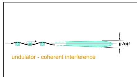
Quasi-monochromatic spectrum with peaks at lower energy than a wiggler  $\lambda_{1} = \frac{\lambda_{u}}{2\gamma^{2}} \left(1 + \frac{K^{2}}{2}\right) \sim \frac{\lambda_{U}}{\gamma_{2}} \text{ (fundamental)}$ + harmonics at higher energy $\epsilon_{1} (\text{keV}) = \frac{0.95 \text{ E}^{2} (\text{GeV})}{\lambda_{u}^{(\text{cm})} \left(1 + \frac{K^{2}}{2}\right)}$  $K = \gamma \theta \text{ where } \theta \text{ is the angle in each pole}$  Synchrotron Radiation Facilities Around the World
