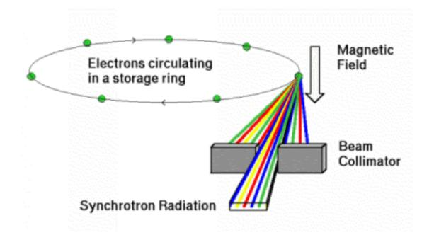
Synchrotron radiation is electromagnetic radiation emitted when charged particles are radially accelerated (move on a curved path).
