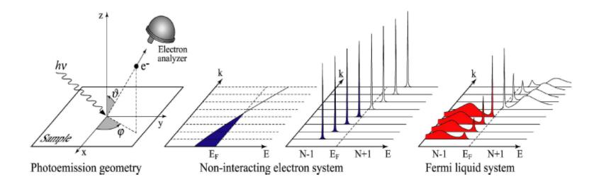
**Photoemission intensity**:  $I(k, \omega) = I_{\theta} |M(k, \omega)|^2 f(\omega) A(k, \omega)$
