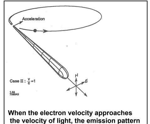
the velocity of light, the emission pattern is folded sharply forward. Also the radiated power goes up dramatically
