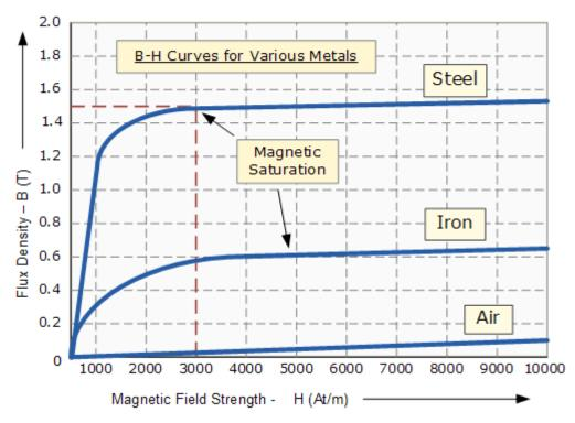
The set of magnetisation curves, M above represents an example of the relationship between B and H for soft-iron and steel cores but every type of core material will have its own set of magnetic hysteresis curves. You may notice that the flux density increases in proportion to the field strength until it reaches a certain value were it can not increase any more becoming almost level and constant as the field strength continues to increase.
