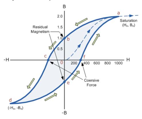
The **Magnetic Hysteresis** loop above, shows the behaviour of a ferromagnetic core graphically as the relationship between B and H is non-linear. Starting with an unmagnetised core both B and H will be at zero, point 0 on the magnetisation curve.
