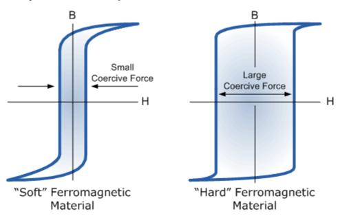
**Magnetic Hysteresis** results in the dissipation of wasted energy in the form of heat with the energy wasted being in proportion to the area of the magnetic hysteresis loop. Hysteresis losses will always be a problem in AC transformers where the current is constantly changing direction and thus the magnetic poles in the core will cause losses because they constantly reverse direction.
