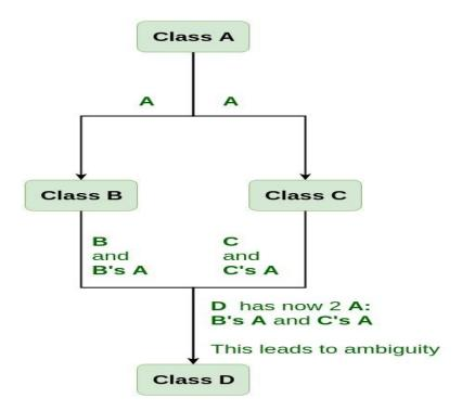
As we can see from the figure that data members/function of class **A** are inherited twice to class **D**. One through class **B** and second through class **C**. When any data / function member of class **A** is accessed by an object of class **D**, ambiguity arises as to which data/function member would be called? One inherited through **B** or the other inherited through **C**. This confuses compiler and it displays error.
