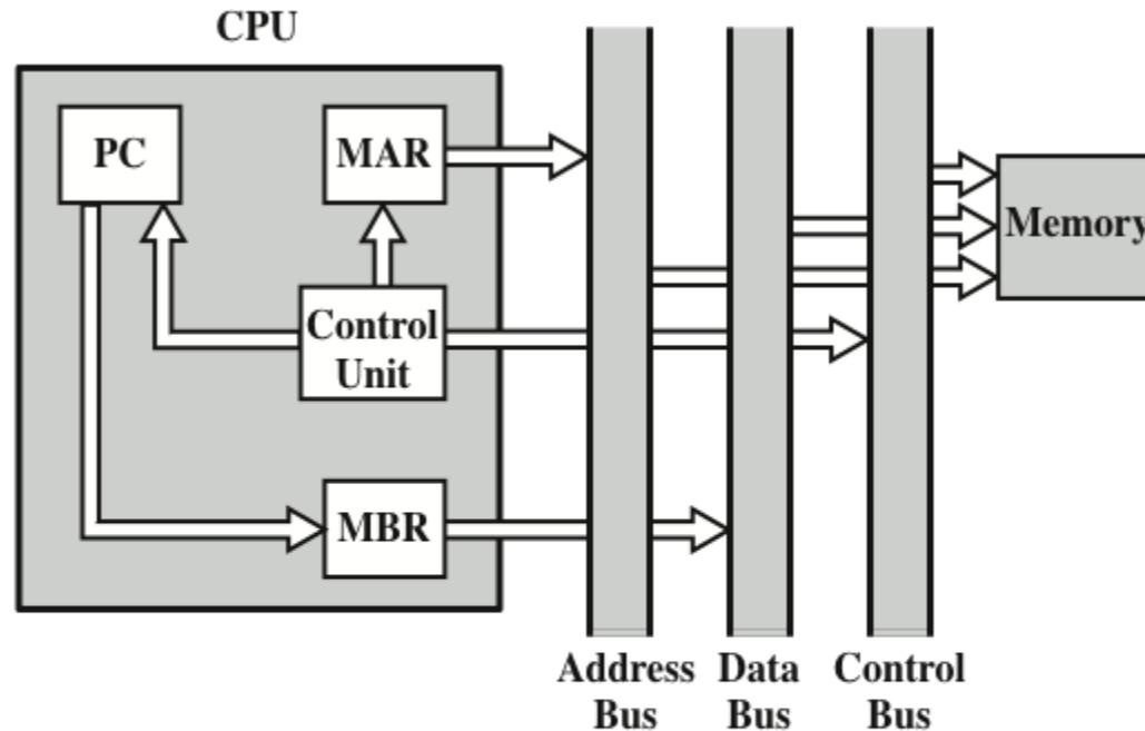
Figure 14.8 Data Flow, Interrupt Cycle
