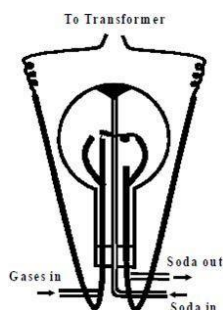
Chemical method for isolation of noble gases
