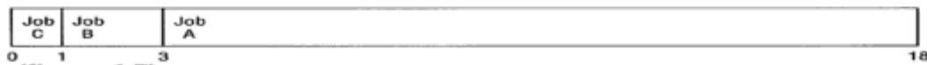
(figure 4.7) Timeline for job sequence C, B, A using the FCFS algorithm. © Cengage Learning 2014
