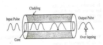
From figure we can see that the pulse received at the output is wider than the input pulse. Hence the output pulse is said to be distorted, due to dispersion effect.
