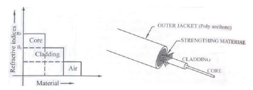
The cladding has low refractive index  $n_2$ . This cladding is covered by a jacket which is made of polyurethane. It protects the layer from moisture and abrasion.
