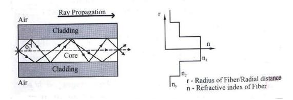
The core is of large diameter. Light follows zigzag paths inside the fibre. Many such zigzag paths of propagation are permitted in Multi-Mode Fibre. The Numerical Aperture of a Multi-mode fibre is larger as the core diameter of the fibre is larger.
