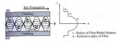
In effect light rays arrive at the end of the fibre are continuously refocused as they travel down the fibre. All rays take the same amount of time in traversing the fibre. This leads to small pulse dispersion.
