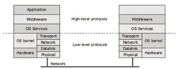
Figure 10-5 Layered organization of a distributed system
