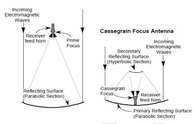
The **angular resolution**, or ability of a radio telescope to distinguish fine detail in the sky, depends on the wavelength of observations divided by the size of the instrument.
