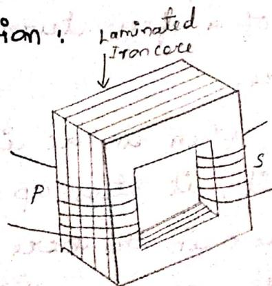
A transformer consists of two coils, called the primary P and secondary S,
