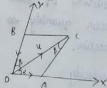
draw  $CA$  parallel to  $oy$ .  $CB$  parallel to  $ox$  making the parallelogram  $DACB$ .
