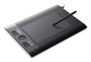
Digitizer is also known as Tablet or Graphics Tablet as it converts graphics and pictorial data into binary inputs. A graphic tablet as digitizer is used for fine works of drawing and image manipulation applications.
