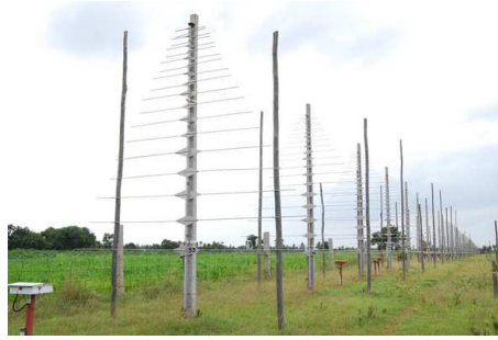
Fig. 5.23 Shows a section of the south arm of the Gauribidanur radioheliograph
