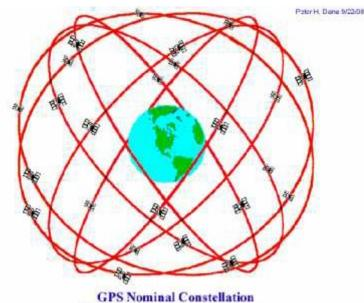
24 Satellites in 6 Orbital Planes 4 Satellites in each Plane 20,200 km Altitudes, 55 Degree Inclination
