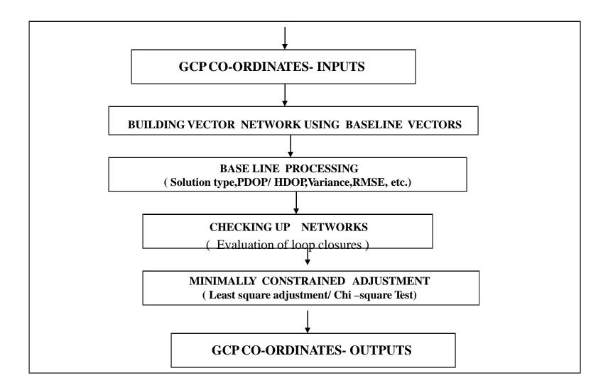
A minimally constrained or free adjustment acts as one quality control check on the network. This adjustment helps to identify bad observations in the network. If an observation does not fit with the rest of the observations , it is highlighted as an outlier.
