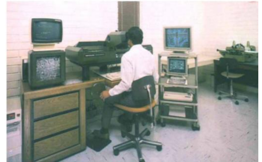
Figure 1-5. Wild BC2 analytical plotter that automates aerial triangulation and simplifies photogrammetric mapping processes. On the table to the right, a point marking and transfer device is shown that drills very small holes in the film emulsion for measurement of pass points and tie points used in aerial triangulation (AT).
