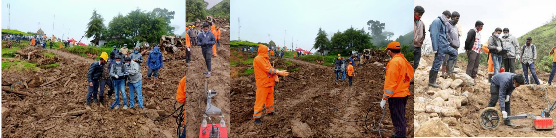
GPR Survey Location 2 Survey Antenna : 200 & 400 MHz No. of Survey lines : 3 Direction : West to East
