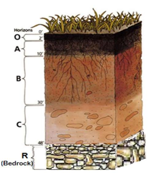
• This sequence of horizons from the surface downwards is called the soil profile. In a typical soil profile following horizons or layers can be recognized.
