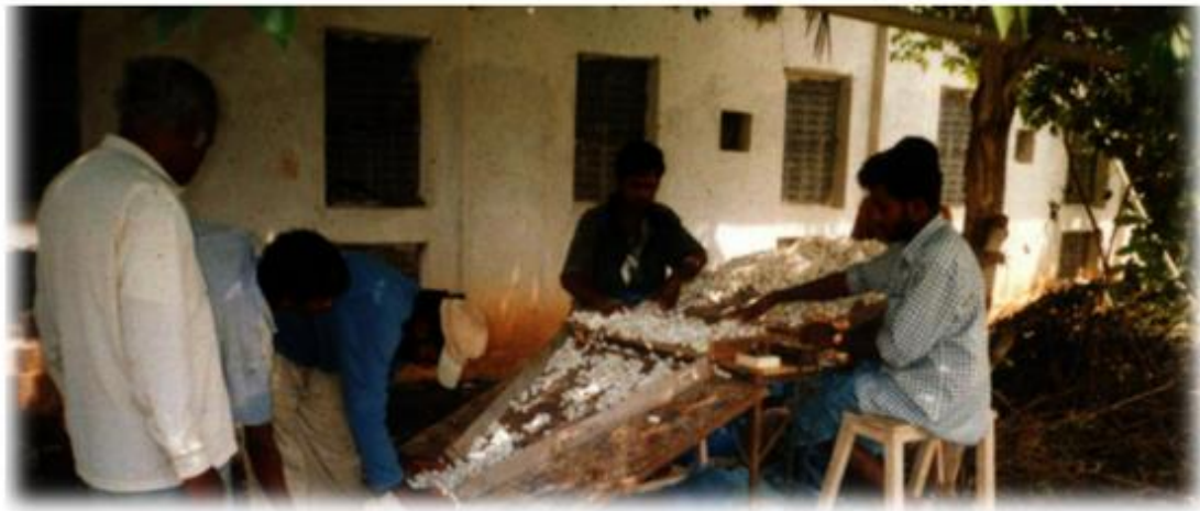
DOUBLE CAPACITY: The machine is simple to operate, portable and can remove about 80 kg of floss a day. Photo: Special Arrangement
