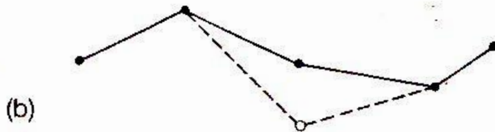
Fig. 8.6 The local nature of splines. When one point is displaced, four intervals must be recomputed for a quadratic spline (a) and two for a linear spline (b).
