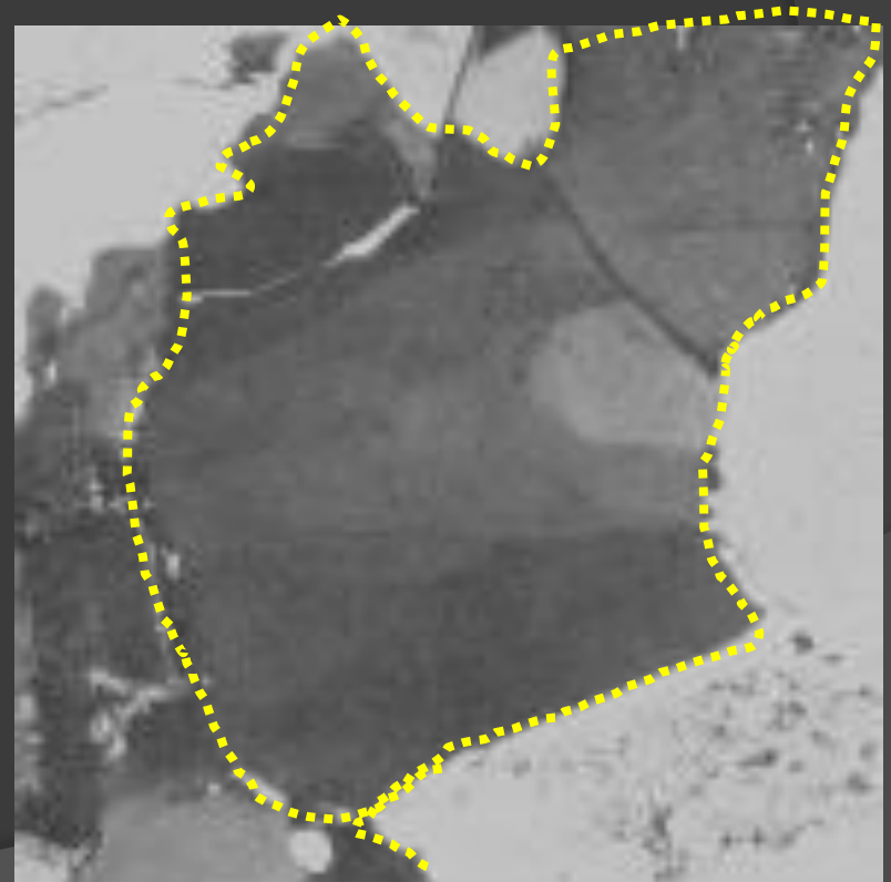
Undulatory Extinction in Quartz
