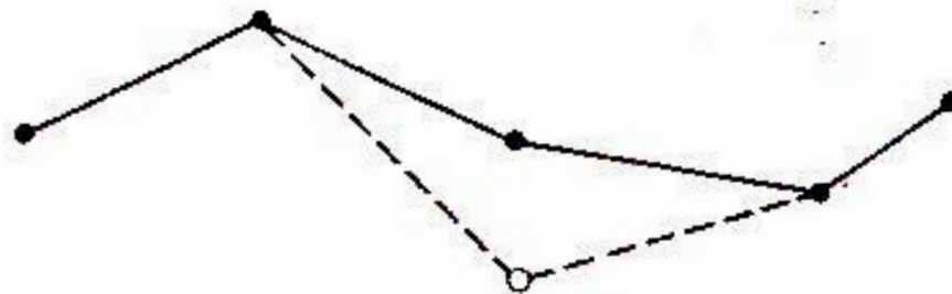
Fig. 8.6 The local nature of splines. When one point is displaced, four intervals must be recomputed for a quadratic spline (a) and two for a linear spline (b).
