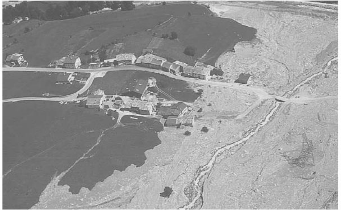
Fig. 4: One of the major flood disasters in the Swiss Alps in 1987 was related to a periglacial debris flow from the Varuna valley (southern Swiss Alps). The debris flow started from a talus slope below Varuna glacier (left image, indicated by circle), damaged the settlement of Privilasco by sediment deposition on the fan (right image), and finally dammed the main river valley. Subsequent flooding caused severe damages of about EUR 30 mill. in the city of Poschiavo (photos: W. Haeberli).
