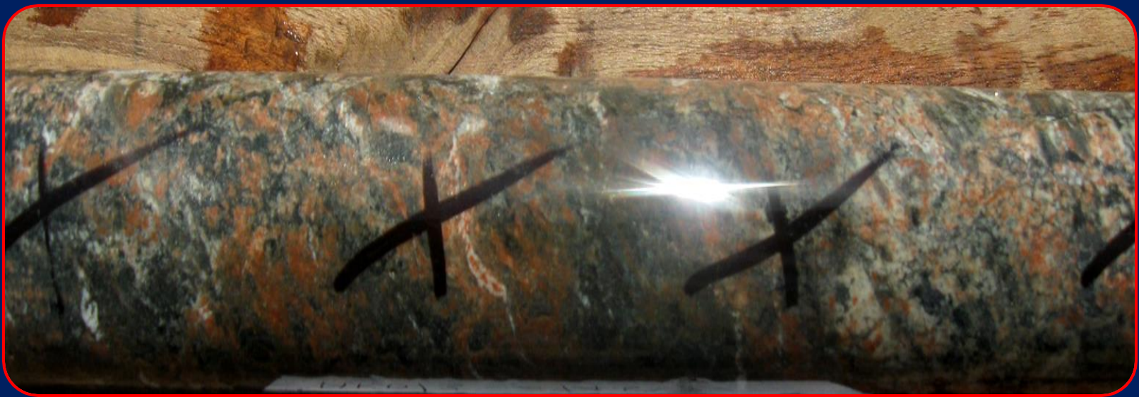
Borehole HKD/3 Radioactive Core showing Albitised Quartz Biotite Schist at 274.50m. Part of mineralised band 0.023 % eU3O8 x 1.90m (274.35-276.25m)
