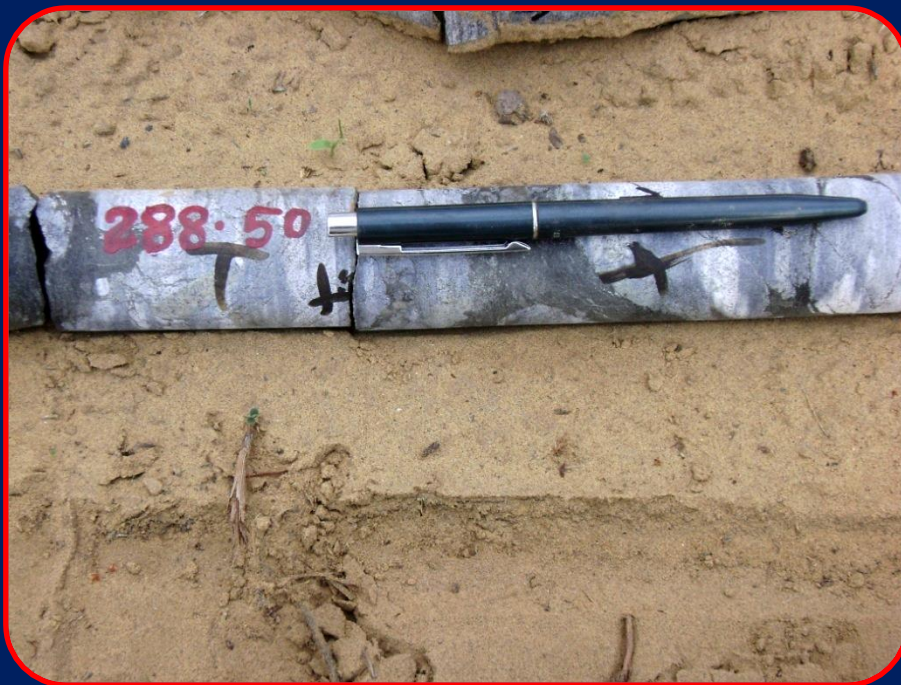
Radioactive Core of Quartzite of RNG-18 at 288.50m (Part of the mineralised band of 0.119x5.70m)
