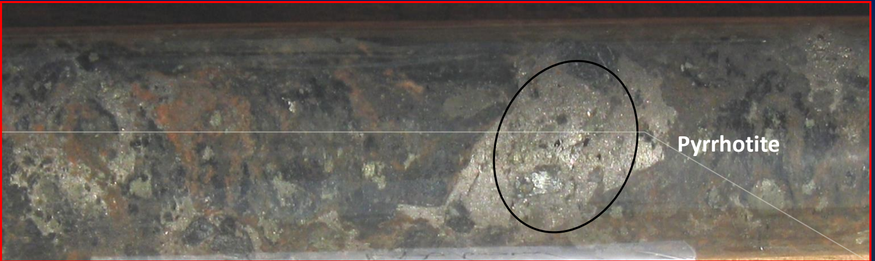
Borehole HKD/2 : Radioactive Core containing chunk of Pyrrhotite at 146.60m. Part of mineralised band 0.144 % eU3O8 x 13.10m (136.25-149.35m)
