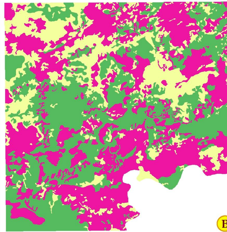
Fig. 18B. - Raster output of Lithology layer Lithology pixel with .415 WOE Value Lithology pixel with -0.95 WOE Value Lithology pixel with -0.13 WOE Value
