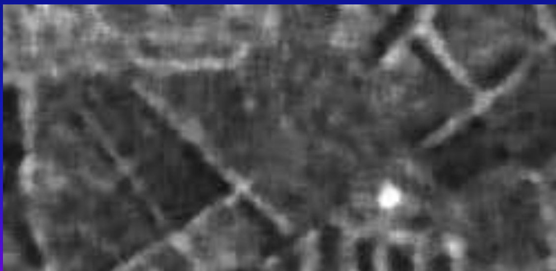
Speckle reduction using an averaging filter
