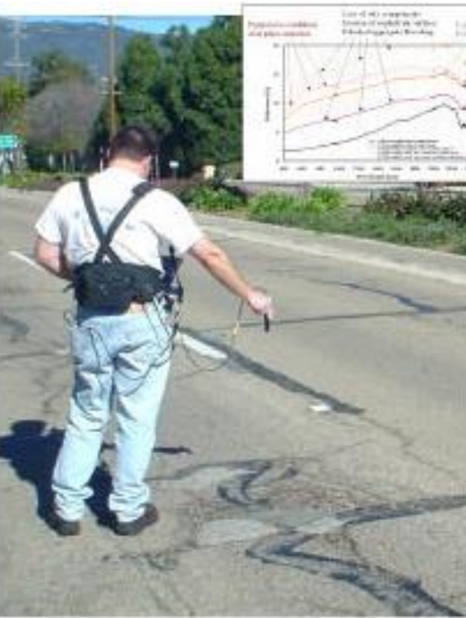
Figure 6: Acquisition of spectral samples of road surface distresses.
